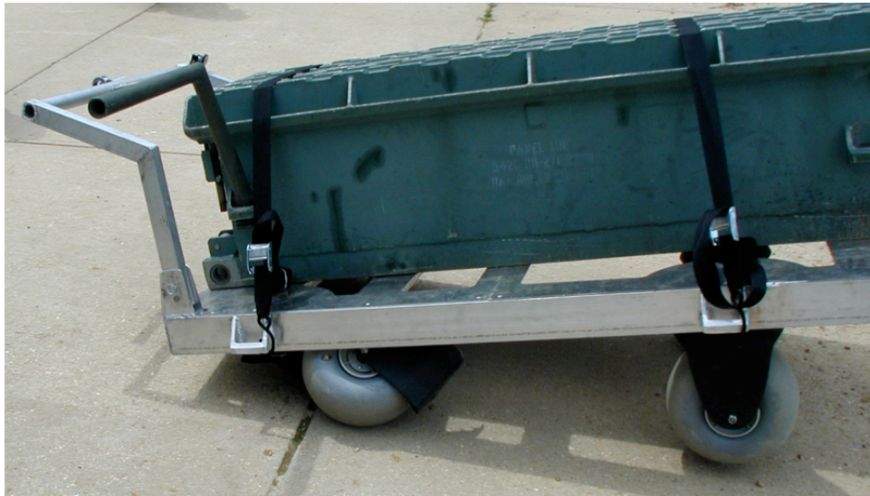
Figure 4.10: Hand Truck Castor Failure
