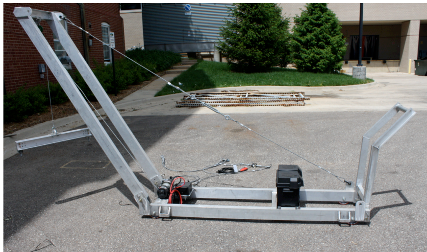
Figure 4.23 Redesigned crane system
