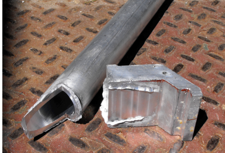
Figure 4.5: Carry Bar Prototype Failure
