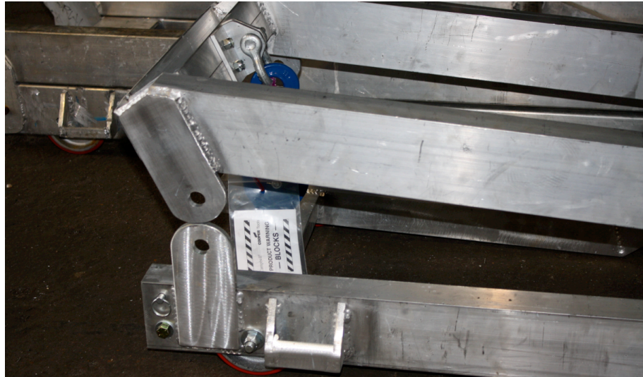
Figure 4.20: Welded Plates for Wire Rope Assembly
